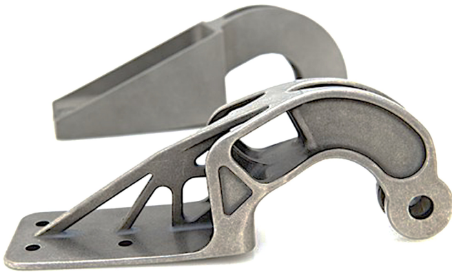
Comparison between brackets made with conventional manufacturing methods (in the back) and with additive manufacturing (in the front).
